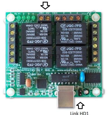
The part numbers for the 5V and 12V versions of the boards will have a -5V or -12V suffix respectively. The 12V variant will also not have the HD1 link option fitted to reduce the possibility of damage if the link was otherwise left fitted.
